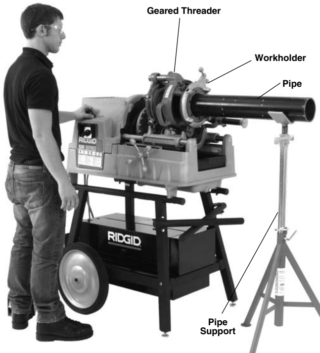
Figure 21 – Operating Position (Close-Coupled Method)
