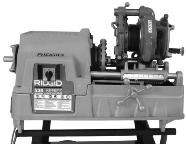
Figure 17 – Geared Threader Close-Coupled To 535
